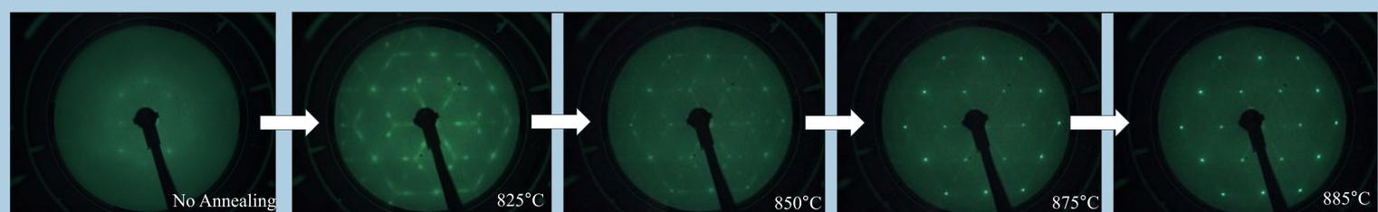
**Stoichiometric  $\text{LiNbO}_3$  demonstrate structural phase transition at temp. over 875 °C to recrystallize to bulk terminated structure with no reconstruction.**
