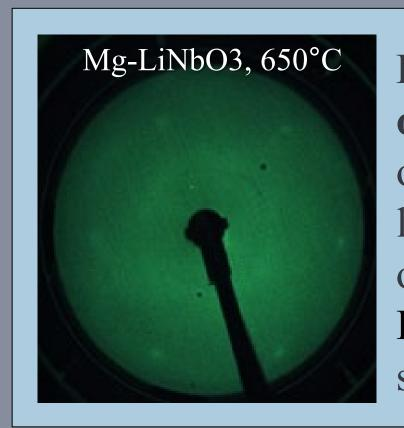
First sign of a LEED pattern at  $650 \,^{\circ}C$ on Mg-LiNbO<sub>3</sub>, exhibiting hexagonal ordered surface crystal structure at the lowest temperature. First sign of an ordered LEED pattern on the undoped LiNbO<sub>3</sub> sample it was at 700°C, for the stoichiometric sample 750°C.
