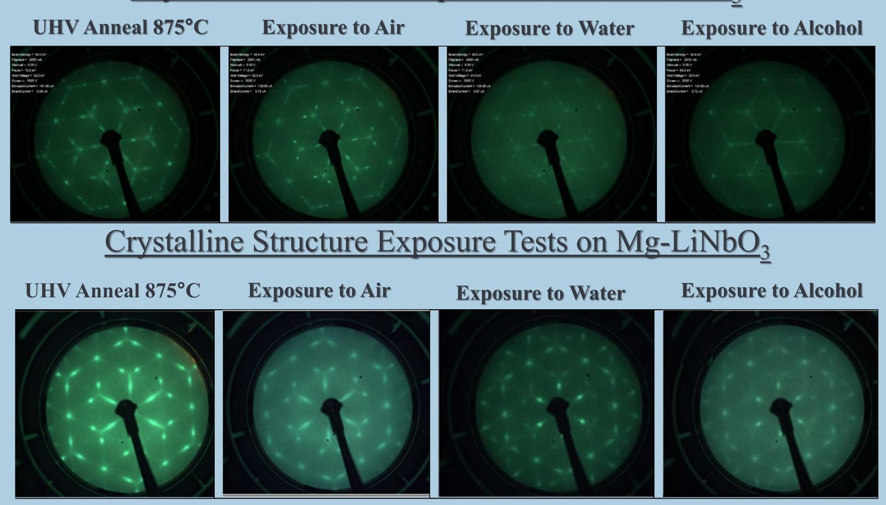
Both the LiNbO<sub>3</sub> and the Mg-LiNbO<sub>3</sub> had no initial LEED pattern before annealing. These samples were annealed in the UHV environment to recover the reconstructed surface crystallography. This crystallography was preserved after exposure to air, water and alcohol with only minor changes.
